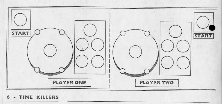
1. Drill or punch the holes marked for buttons or bolts. Use a chassis or sheet metal punch for best results on button holes.
