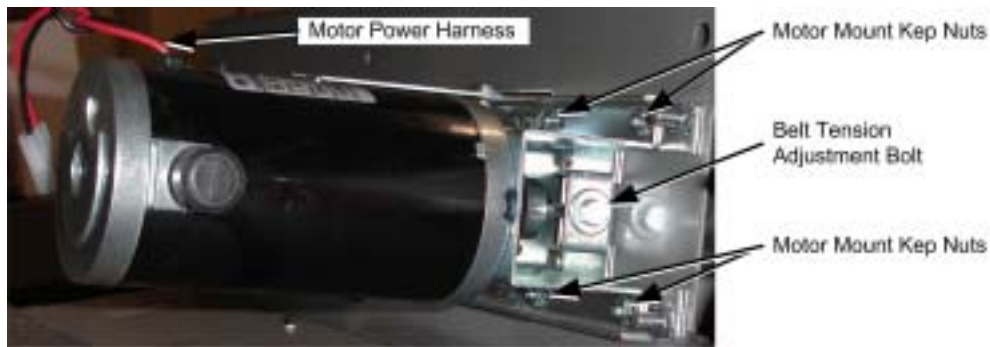
Figure 31. Servicing the Steering Motor
