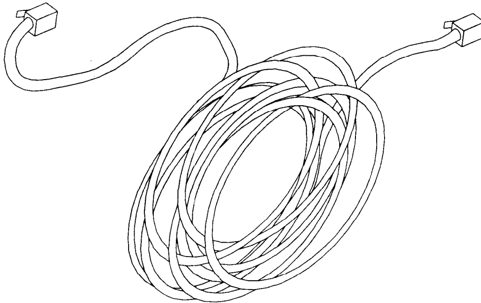
LINKING CABLE (UNSHIELDED TWISTED PAIR CATEGORY 5)
