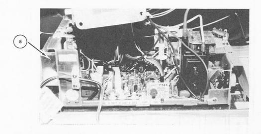
Hot Rod Printed Circuit Board
