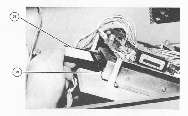
REMOVE THE LID of the SHIELD CASE. Remove the sheet metal and pull out the game board unit in a manner so that both ends of it will meet the shield case. Open the FDD (Floppy Disk Drive) LID by taking off the 2 (M3 x 8) SCREWS when replacing the FLOPPY DISK.
